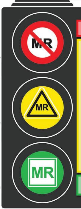
and other equipment used in or near the MR environment should be labeled as MR Unsafe, MR Conditional, or MR Safe.
